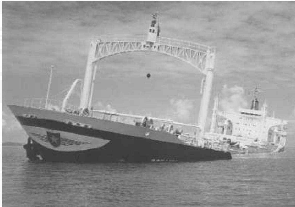
Figure C.6: Oceanic Grandeur after flooding. Hull is under extreme sagging moment but survived. No new tanker would. Note the extremely strong kingposts and the rare forward crowsnest, signs of an unusually well-specced ship. Source: Australian Maritime Safety Authority.
