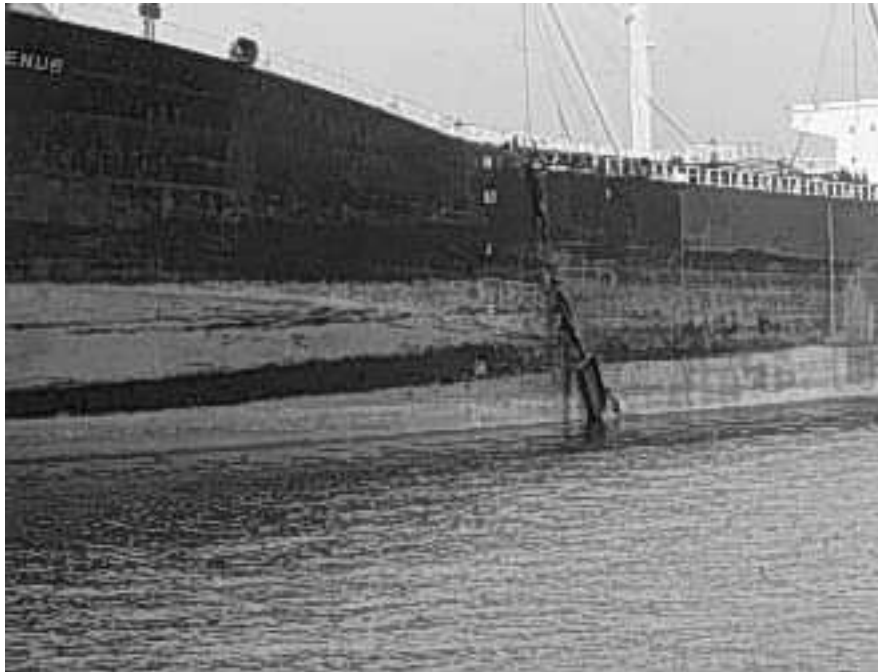
Figure 3.3: Alvenus buckled after grounding. Source: R. Hann.
