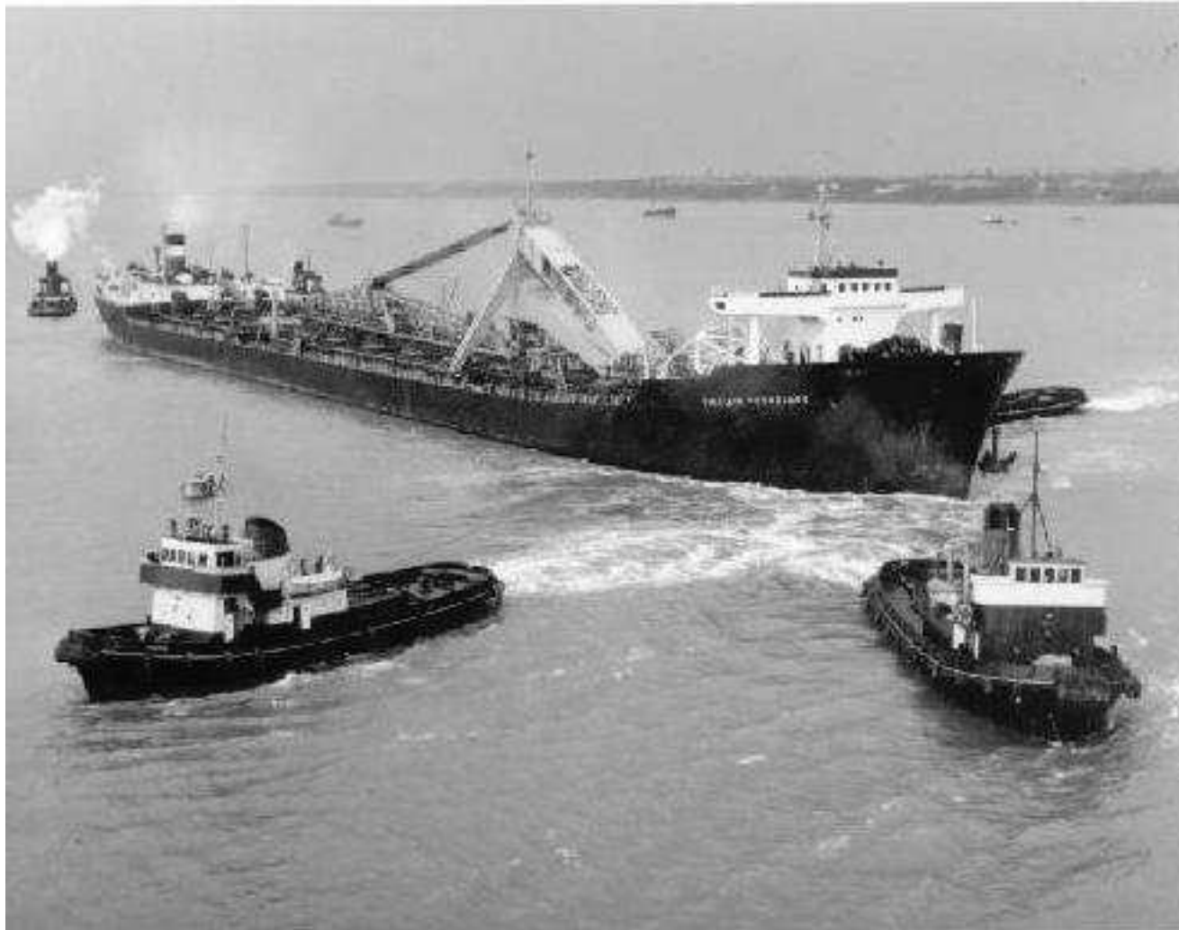
Figure 2.2: Sinclair Petrolore: Self-Unloading Ore-Oil Carrier. Source: www.solentwaters.co.uk
