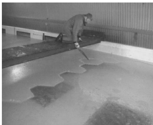
Fig. 3. The floes were cut manually by use of saw.
