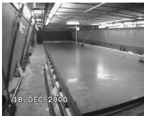
Fig. 1. The test basin seen from the melt basin end. The ceiling was about 2.5 m above the ice cover.
