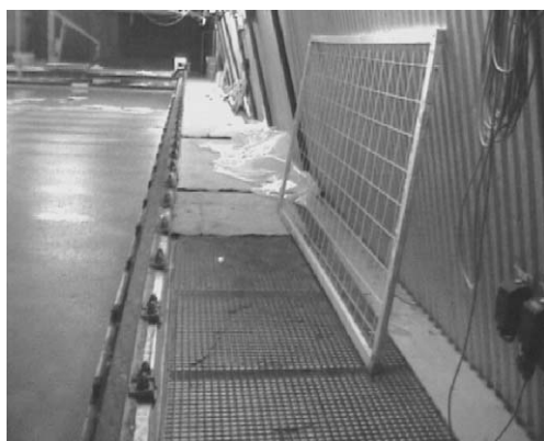
Fig. 8. Grid used to correct the images. The outer dimensions for the wooden frame are 1.5 × 3 m and the squares are 15 × 15 cm.
