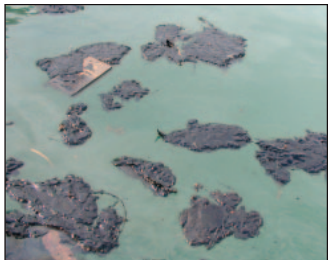
Oils spilled into the sea at temperatures below their pour point form solid fragments. This photo shows Nile Blend crude, pour point +33° C, in sea water of 28° C. Such oils are highly persistent and have the potential to travel great distances.
