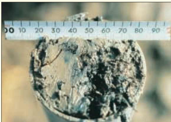
Cross section of core at 10 cm depth from mudflat showing penetration of oil
